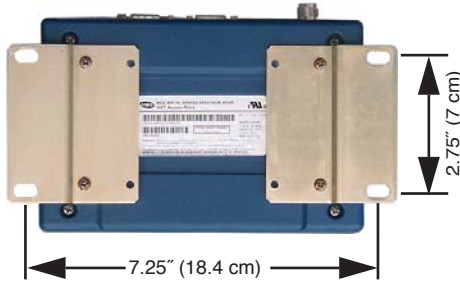
Figure 1. AP Mounting Bracket Spacing
