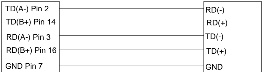
Figure 5. RS-422/RS-485 (Four Wire) Pinout Description
